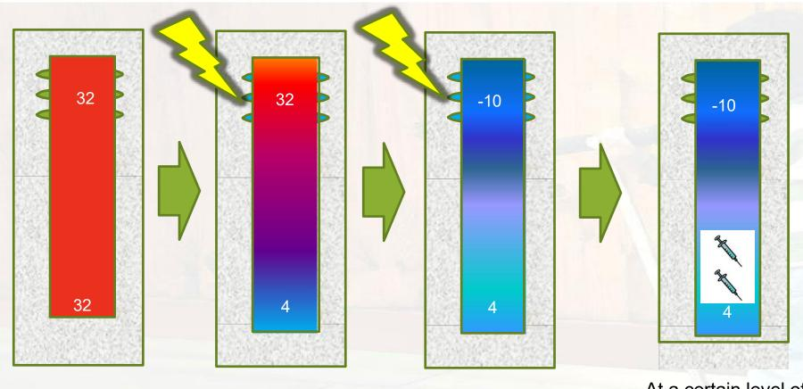
Water @ Ambient temp Cooling induced. Water @ 4 deg denser, settles down
